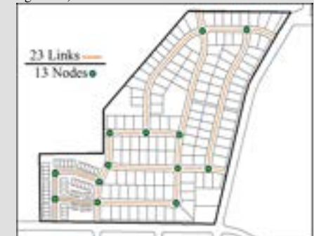
Figure 27. Example connectivity index calculation showing nodes and links. This example shows 23 links and 13 nodes which equates to a connectivity index of 1.77.
