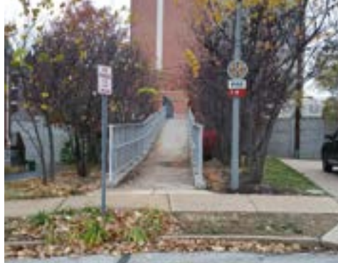
Examples of pedestrian and bike connections through property barriers at the ends of cul-de-sacs or through a large block.
