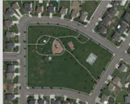
Figure 31. Park layout allows access from all sides with home fronts facing the park.
