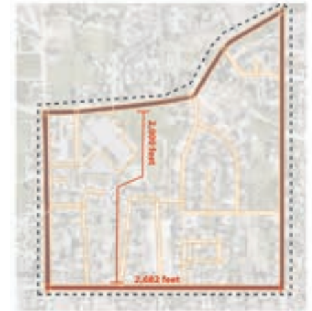
The diagram on the right shows the measurement of two of the longest pedestrian blocks, or “gaps” between links in the pedestrian network.
