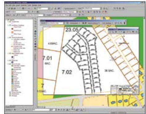
ArcScan™ for ArcGIS—Converts raster scans of parcel maps into vector-based geodatabase feature classes. ArcPress for ArcGIS helps produce high-quality maps quickly.
